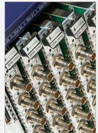
Close-up view of the rear of a HCU1500 showing RPM2000 modules.
