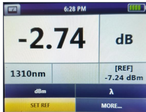
Figure 5: Optical Insertion Loss Results
