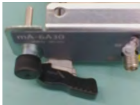
Figure 7-1 Securing Latch - Locked Position
