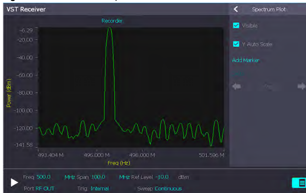
Figure 6-14 Receiver Spectrum Plot Panel
