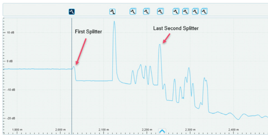
Figure 6 – OTDR trace between 1st splitter and last 2nd splitter
